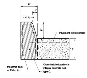
INTEGRAL CONCRETE CURB TYPE C (BARRIER)
