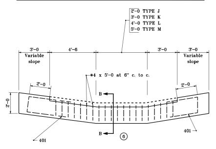
**ELEVATION VIEW** LUG FOR PAVED SIDE DITCH TYPES J THROUGH M
