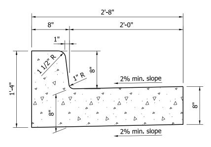
COMBINED CONCRETE CURB AND GUTTER, TYPE C (VERTICAL)
