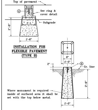
INSTALLATION OUTSIDE OF PAVEMENT (TYPE C)
