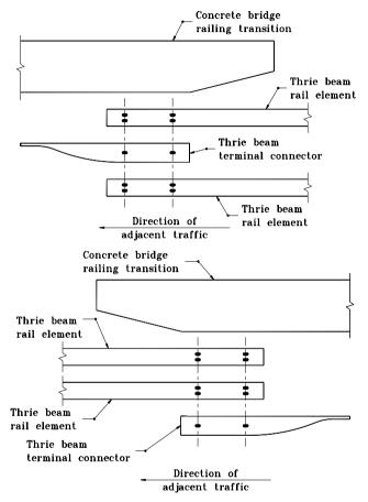
LAP DETAIL AT BRIDGE RAILING TRANSITION
