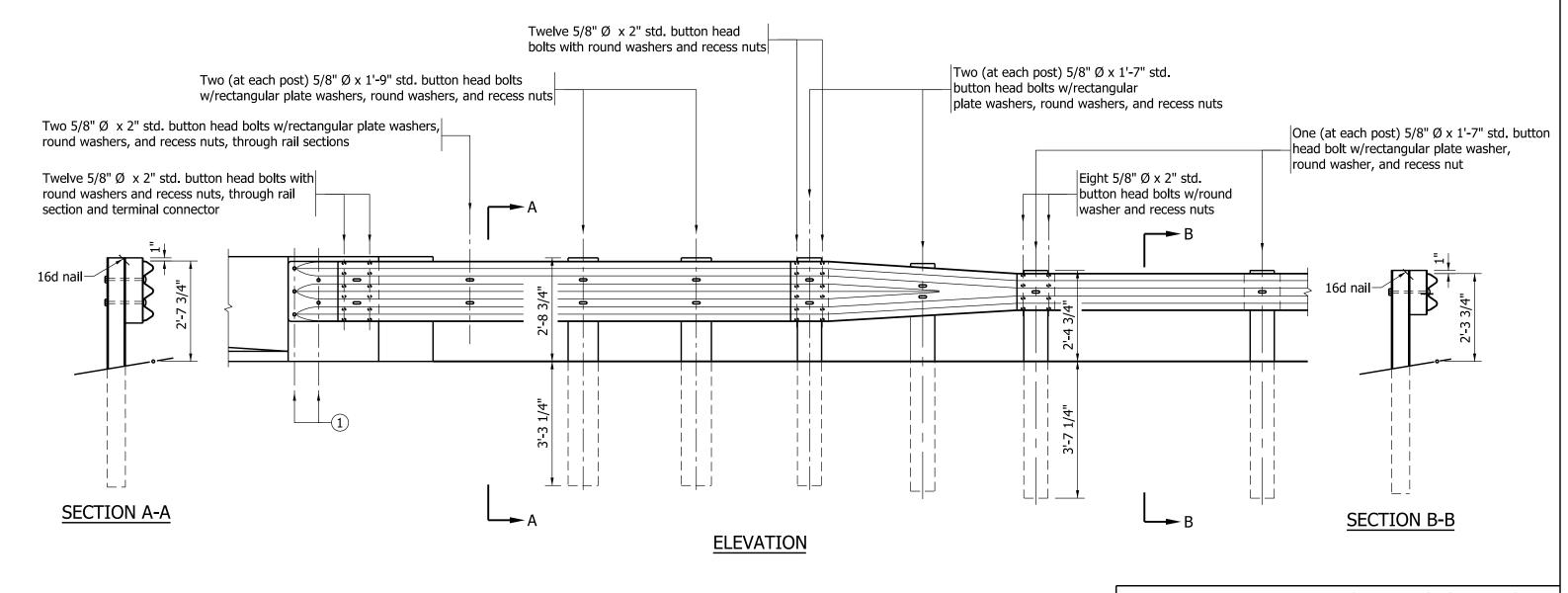
① See pier connection details for connection of terminal connector. See Standard Drawing E 601-TTGP-01 (use proper end detail).
