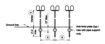
**SPACING FOR MULTIPLE POST INSTALLATION**
