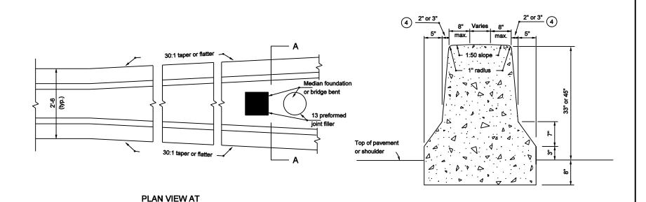
INTEGRAL MEDIAN FOUNDATION OR BRIDGE BENT
