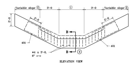
LUG FOR PAVED SIDE DITCH TYPES E THROUGH H
