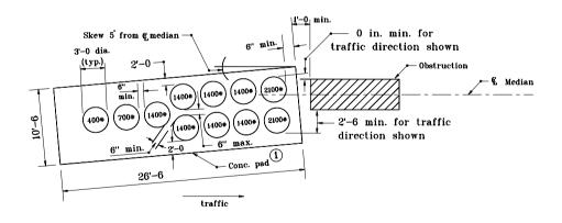
CONCRETE PAD PLAN IMPACT ATTENUATOR TYPE ED GRAVEL BARREL ARRAY FOR TEST LEVEL 2
