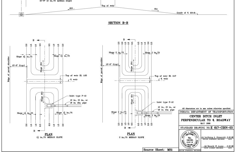
① See Standard drawing MS for inlet type P-12 details.
