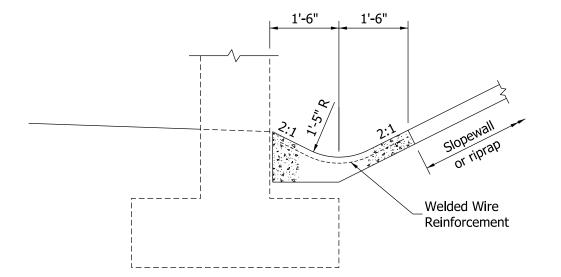
SECTION THROUGH PAVED DITCH AT TOE OF SLOPE (See layout on plans for location of paved ditch)
