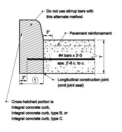
ALTERNATE METHOD OF CONSTRUCTION FOR ALL TYPES OF INTEGRAL CONCRETE CURB
