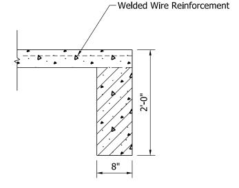
SECTION A-A TYPICAL ELEVATION THRU SLOPEWALL
