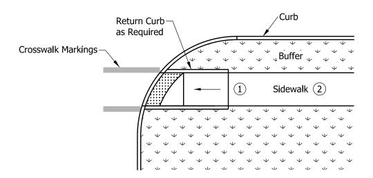
ONE-WAY DIRECTIONAL PERPENDICULAR CURB RAMP WITH BUFFER
